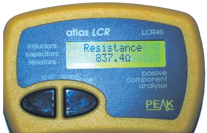
Resistance measurement readout.
