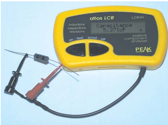
Checking-out the value of a suspect electrolytic capacitor.
