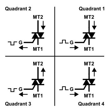
The main load current is handled by the connections MT1 and MT2. The device is switched to the on state by a current into (or out of) the gate terminal with respect to the MT1 terminal.
