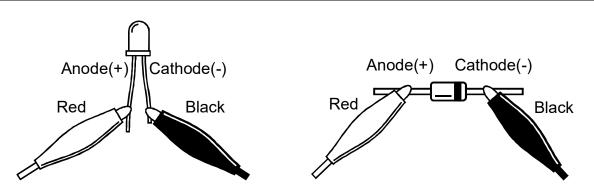
The Anode(+) of the LED or diode should be connected to the red probe. The Cathode(-) of the LED or diode should be connected to the black probe.
