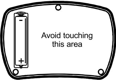
We recommend that the battery is replaced with a high quality battery equivalent to an **AAA Alkaline or Lithium-Iron-Disulphide**, LR03 or MN2400 (1.5V). Replacement Alkaline AAA batteries are available from many retail outlets.
