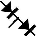
Here, each diode is connected in series. An example is the BAV99.
