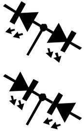
3-lead bicolour LEDs are available in common cathode and common anode varieties. The **DCA Pro** supports both types.
