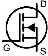
MOSFET stands for *Metal Oxide Semiconductor Field Effect Transistor*. They are available in two main types, N-Channel and P-Channel. Most modern MOSFETs are of the Enhancement Mode type, meaning that the bias of the gate-source voltage is always positive (For N-Channel types). The other (rarer) type of MOSFET is the Depletion Mode type which is described in a later section.
