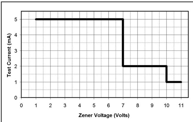
\*The **DCA Pro** may not be able to identify Zener diodes with a Zener voltage of more than 11V. It will however still identify the diode junction in its forward biased mode.
