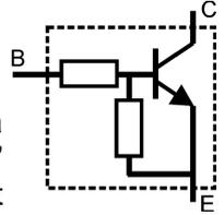
These transistors are usually found in surface mount packages and are becoming more common, particularly in mass produced electronic products.
