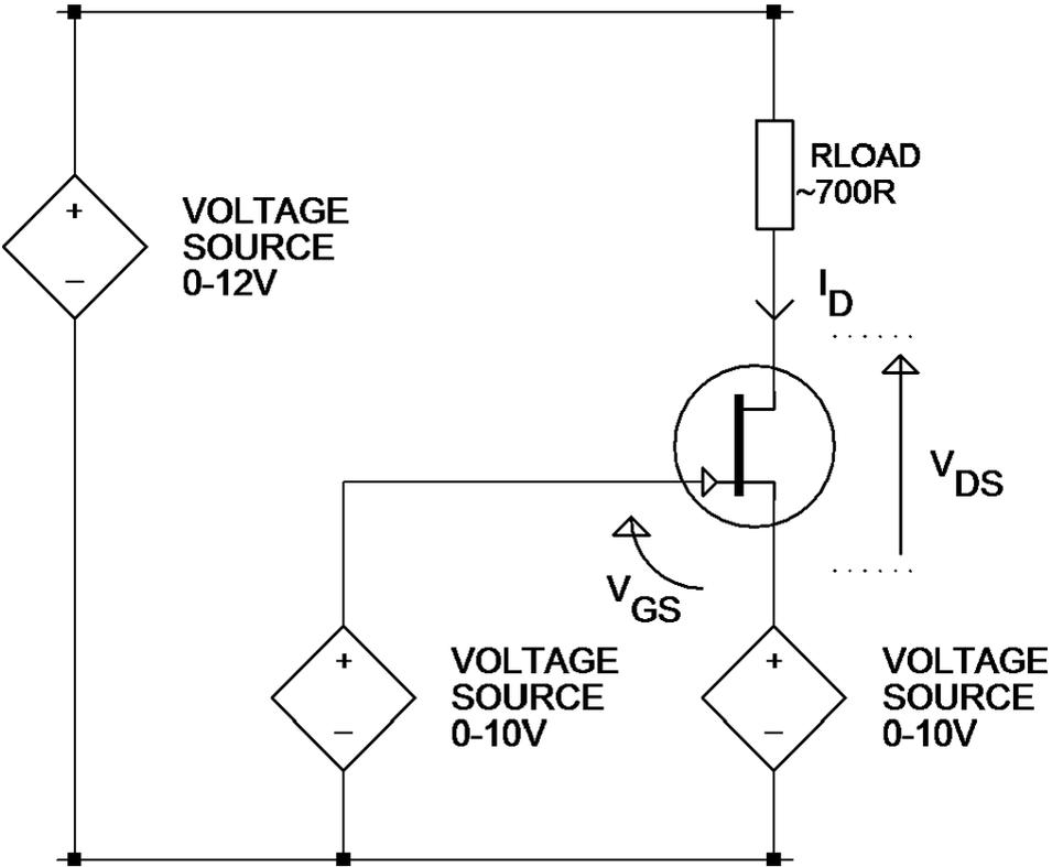
It's important to note that the gate-source voltage can be driven negative by making the source voltage drive higher than the gate voltage drive. When this is done however, there is less voltage available to be across the drain-source nodes and the load resistor.
