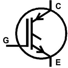
Like MOSFETs, IGBTs are available as enhancement mode and depletion mode types.
