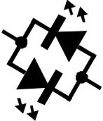
Bicolour LEDs are generally available in two main varieties; 2-lead and 3-lead types.
