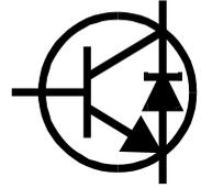
If a free-wheeling diode has been detected, it is shown on the schematic symbol. Some examples are shown here:
