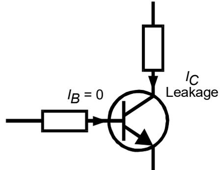
$I_{CLeak} = 0.177\text{mA}$
