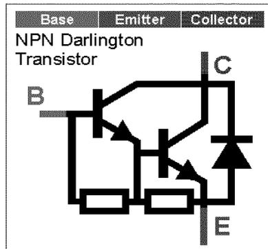
Note that the component schematic is displayed in colour to illustrate which colour test lead is connected to each component lead.
