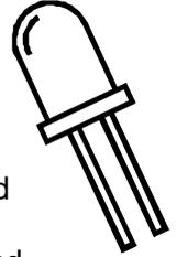
An LED (light emitting diode) is really just another type of diode, however, the **DCA Pro** will determine that an LED or LED network has been detected if the diode's measured forward voltage drop is between 1.5V and 4.0V. This also enables the **DCA Pro** to intelligently identify bicolour LEDs, both two-lead and three-lead varieties. See the section on bicolour LEDs for more information.
