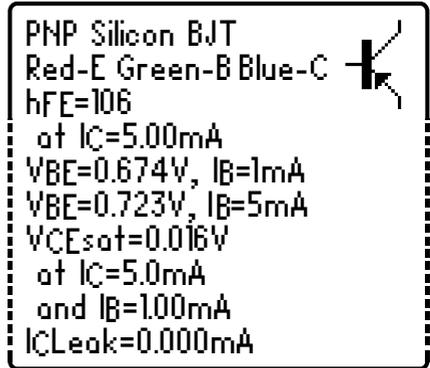
This example shows that the Red test clip is connected to the Emitter, the Green is connected to the Base and the Blue test clip is connected to the Collector.
