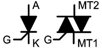
Thyristor terminals are the anode (A), cathode (K) and the gate (G).
