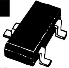
The **DCA Pro** will identify multiple diode junctions between the probes. For three terminal devices such as SOT-23 diode networks, all three test clips must be connected. The optional Peak Component Adapter for SOT-23 parts (Peak model PCA23) can be useful for testing SOT-23 parts.
