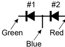
In the same way as the single diode analysis, the forward voltage for each diode is measured for a nominal test current of 5mA.
