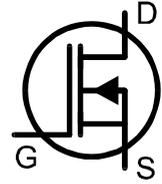
The fairly rare Depletion Mode MOSFET is very similar to the conventional Junction FET (JFET) except that the gate terminal is insulated from the other two terminals. The input resistance of these devices can typically be greater than 1000MΩ for negative and positive gate-source voltages.
