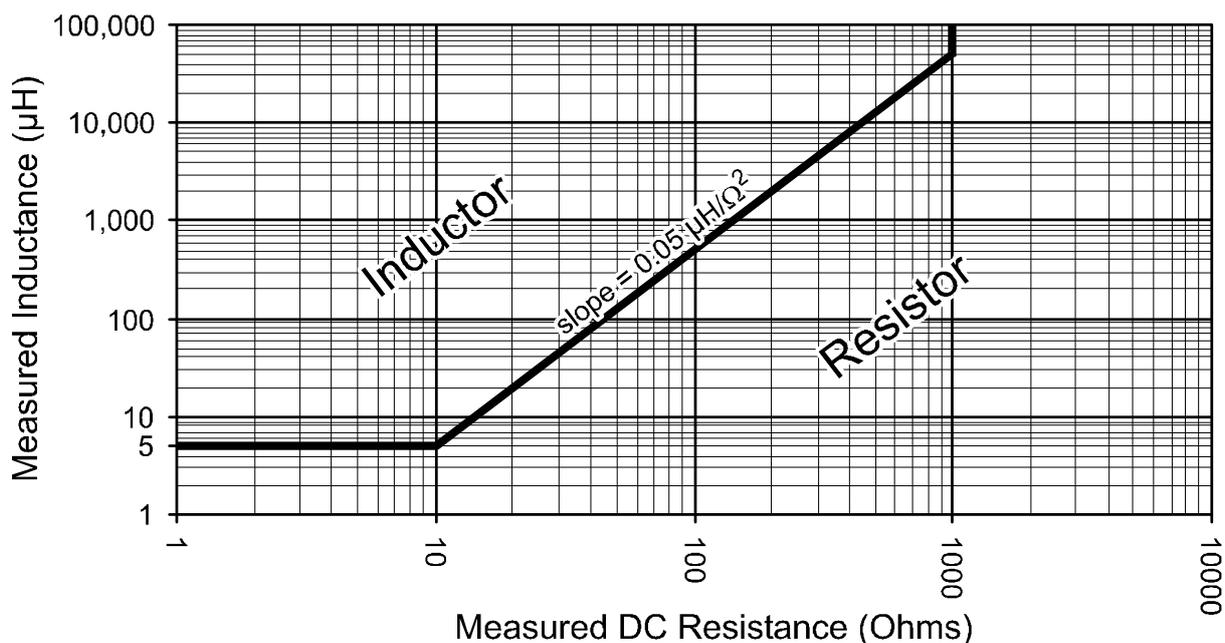
For example, if the inductance of your component is measured at 100µH and it has a DC resistance of 100Ω, then the **LCR40** will tell you that you have a resistor. If however the resistance was only 10Ω, then the **LCR40** will tell you that you have an inductor.
