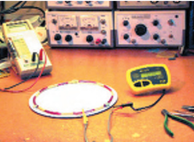
Checking the inductance of a metal detector pulse induction search coil
