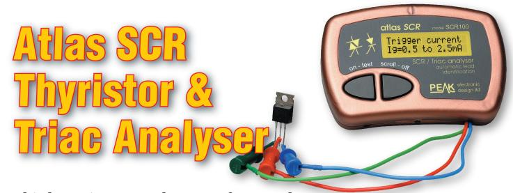
This latest in-your-palm tester from Peak will reliably check all thyristors and Triacs that you are likely to encounter. Just connect the mini-hook leads (in any order) and press "test"!
