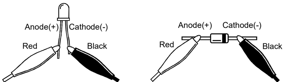
The Anode(+) of the LED or diode should be connected to the red probe.
