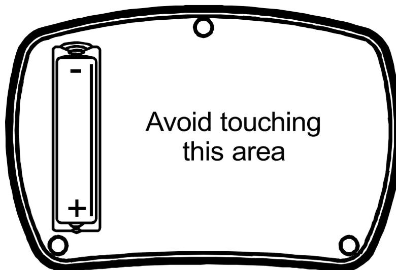
We recommend that the battery is replaced with a high quality battery equivalent to an **AAA Alkaline or Lithium-Iron-Disulphide**, LR03 or MN2400 (1.5V). Replacement Alkaline AAA batteries are available from many retail outlets.
