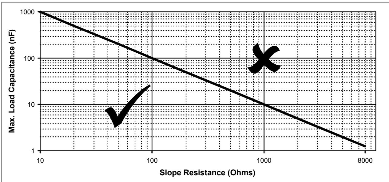
**Resistive Loading** - Depending on the selected test current range, the following resistive loads will influence  $V_z$  measurements by 1% or more:
